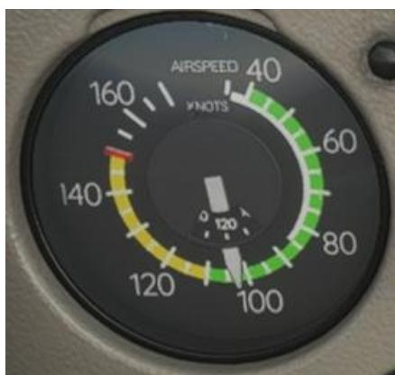
The airspeed indicator is essentially a pressure gauge. The harder the air is hitting the aircraft, and flowing into the Pitot Tube, the higher the reading, which is calibrated to display Nautical Miles Per Hour (Knots). As discussed in principles of flight, the speed of the air going past the wing is directly related to the lift produced.
