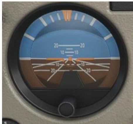
Whilst your primary flying reference when VFR is the horizon, fine adjustments and precise attitudes can be obtained by use of the AI. Of most interest for visual flight is the angle of bank markings along the top. The first 3 white lines either side of centre designate 10 degrees of bank each, until the fourth line which indicates 60 degrees. Normal turns will be made at about 20 degrees.
