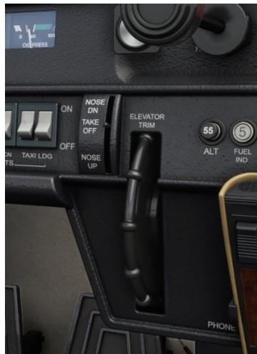
The most common method of providing trim control on light aircraft is with the trim tab. This is a small control surface at the trailing edge of the elevator which is moved independently with trim wheel control in the cockpit.
