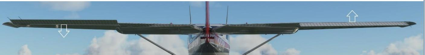
Simultaneously the right aileron is lowered, increasing lift on the right wing. These two lift adjustments combine to roll the aircraft to the left.
