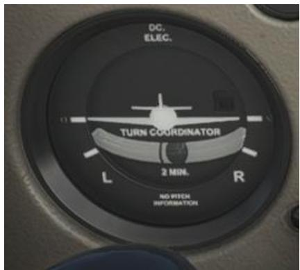
For VFR flight, the slip indicator on the turn coordinator is used throughout the flight to guide the pilot which inputs to make with the rudder. Keeping the black ball centred in the gauge ensures the aircraft is correctly aligned into the oncoming airflow, which gives the least drag and maintains passenger comfort.
