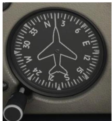
The DG is your primary reference for flying particular headings. As the DG is gyroscope powered, gyroscopes can drift over time and lose accuracy. Before departure and periodically in flight you will check that the DG heading agrees with the magnetic compass and make any adjustments necessary.
