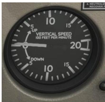
The VSI is useful for accurately ensuring level flight, but does often have some lag to it. Also, a pressure instrument, the VSI senses rate of altitude change and displays in Feet Per Minute (FPM).
