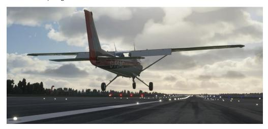
At the appropriate moment you'll turn right onto a heading of South to fly the 'base leg'. Simultaneously reduce power and lower the nose slightly to begin a gradual descent. Once the speed has come back to within the white band on your ASI, you can extend the first 10 degrees of flaps.
