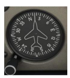
The DG is your primary reference for flying particular headings. As the DG is gyroscope powered, gyroscopes can drift over time and lose accuracy. Before departure and periodically in flight you will check that the DG heading agrees with the magnetic compass and make any adjustments necessary.
