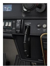
The most common method of providing trim control on light aircraft is with the trim tab. This is a small control surface at the trailing edge of the elevator which is moved independently with trim wheel control in the cockpit.
