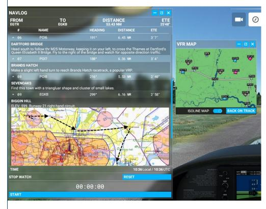
Navigate enroute with the NavLog, which includes your Heading, Distance and Estimated Time Enroute (ETE) for each waypoint.
