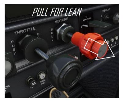
If too much fuel is being supplied, the fuel/air mixture is termed as 'rich', which is experienced as a loss of performance. Prolonged rich running wastes fuel and can also cause carbon build-up in the engine, decreasing performance further and causing rough running.
