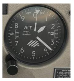
Indicating your altitude in thousands of feet, the altimeter is read in the same way as a clock, with a short (hour) hand and a long (minutes) hand. The short hand indicates thousands of feet, the little indicates hundreds.
