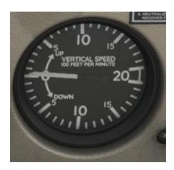
The VSI is useful for accurately ensuring level flight, but does often have some lag to it. Also, a pressure instrument, the VSI senses rate of altitude change and displays in Feet Per Minute (FPM).
