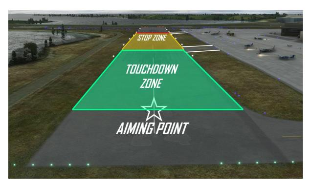
For this landing onto runway 24, use the middle of the first centreline stripe as an aiming point. Strive to touchdown in the zone shown in green, between the aiming point and the first taxiway on the right.
