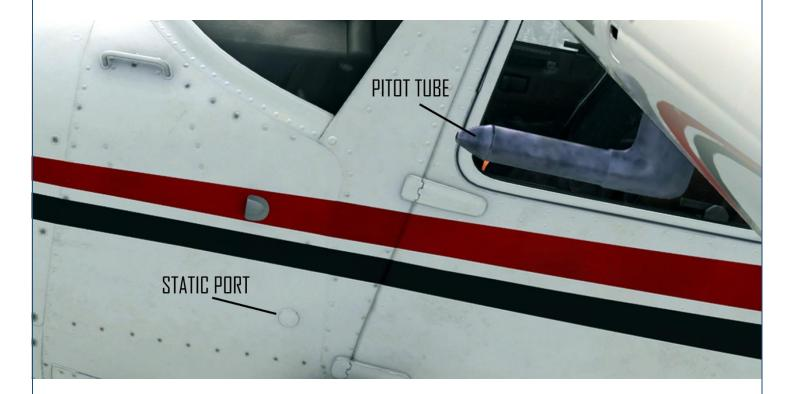
The Airspeed Indicator (ASI) has two sources of air pressure. Like the altimeter and VSI, the ASI is supplied with static pressure. The ASI is also fed with 'ram air' which is provided by the pitot tube. Ram air is the total oncoming airflow that enters the pitot tube. By subtracting the static pressure from the ram air, we get 'dynamic pressure' which the ASI is calibrated to display as an Indicated Airspeed (IAS).
